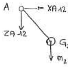
$$\begin{cases} X_{A12} \vec{x}_2 + Z_{A12} \vec{z}_2 + m_2 g \vec{z}_2 = m_2 \vec{\Gamma}_{G_2/Rg} \\ \vec{A}_{G_2} \wedge m_2 g \vec{z}_2 = \vec{A}_{G_2} \wedge m_2 \vec{\Gamma}_{G_2/Rg} \end{cases}$$
