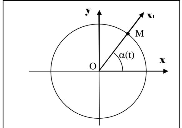
**$\mathbf{OM} = R \mathbf{x}_1$  ;  $\mathbf{V}(M/R) = a \alpha^\circ(t) \mathbf{y}_1$  ;  $\mathbf{\Gamma}(M/R) = a \alpha^{\circ\circ}(t) \mathbf{y}_1 - a \alpha^{\circ 2}(t) \mathbf{x}_1$**
